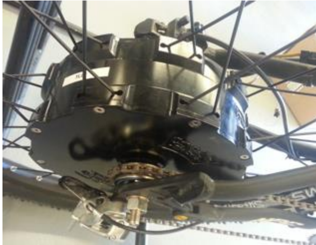
3600 W kit motor. Source: https://www.electricbike.com/12-kit-power-levels-360w-to-8000w/
