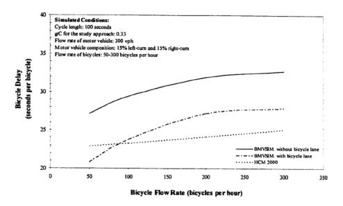
Figure 2-1: Bicycle delay against bicycle flow rate (Raksuntorn 2002)
