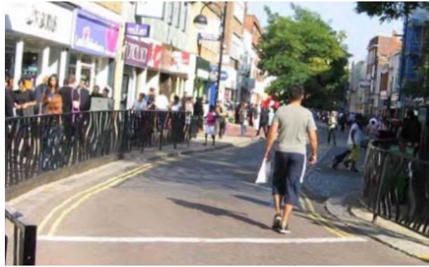
Figure 4: People may walk on the road if frequent barrier gaps are not provided (Hounslow, London)
