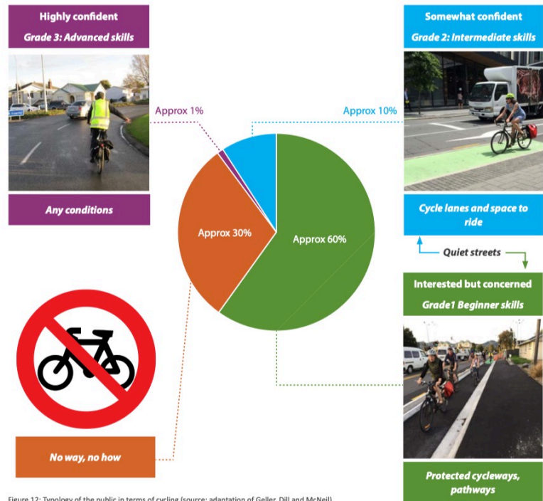
Figure 12: Typology of the public in terms of cycling (source: adaptation of Geller, Dill and McNeil)
