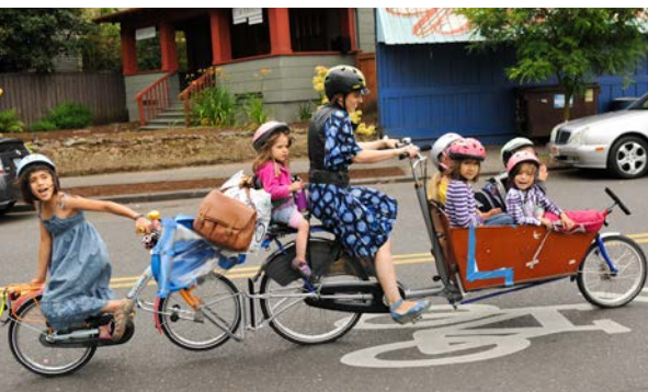
Figure 3: A cargo bike with child seat and tag-along (Image copyright Jonathan Maus)
