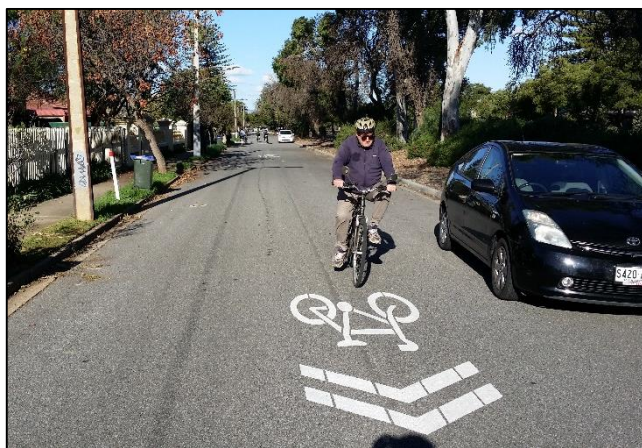
Figure 19: Sharrows on a quiet street, Adelaide, Australia
