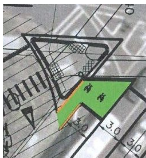
Figure 8: Revised scheme – reassigned lane dimensions
