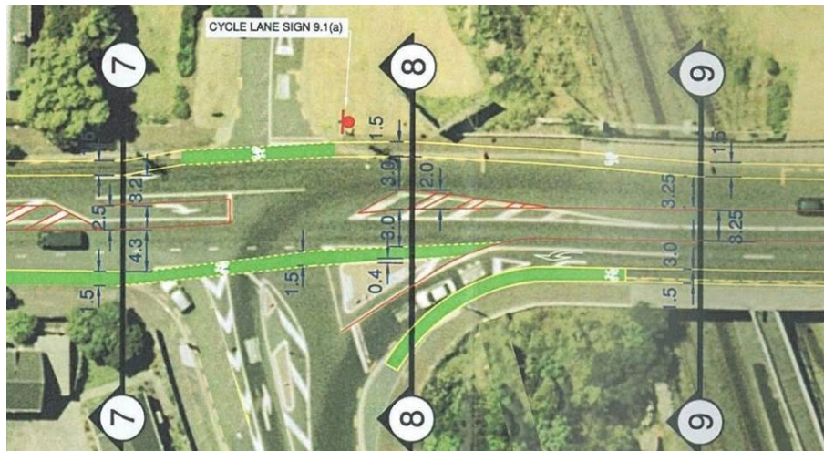
Figure 5: Discontinuous cycle lane across left turn slip lane in old scheme
