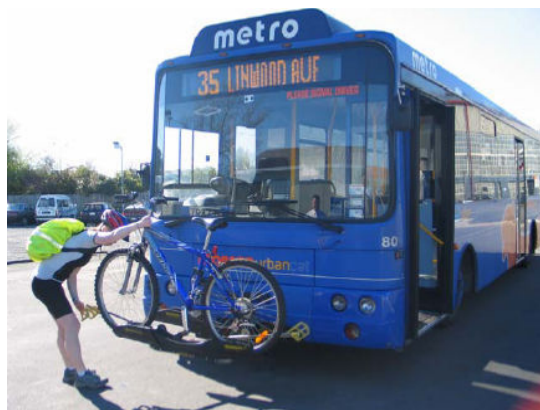
Figure 16: Bike racks have been installed on Christchurch to Lyttelton buses allowing cyclists to travel through the Lyttelton Tunnel
